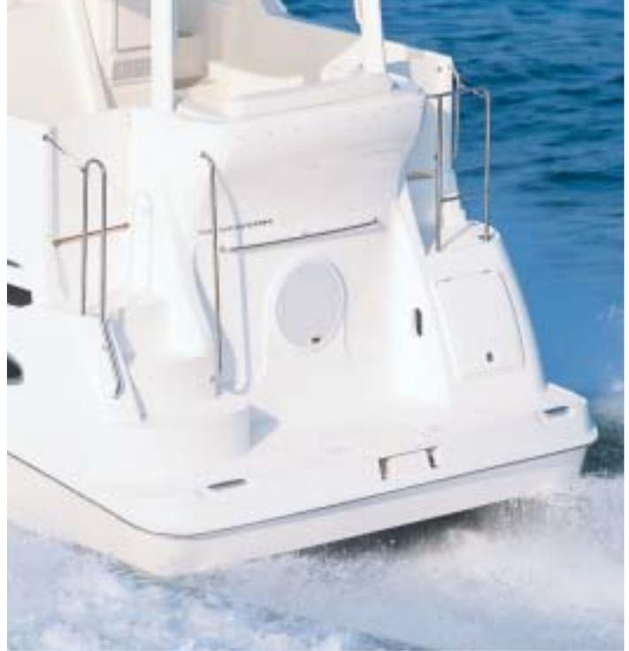
*Wide, molded-in steps and sturdy stainless steel handrails make moving around the boat safe and easy.*
