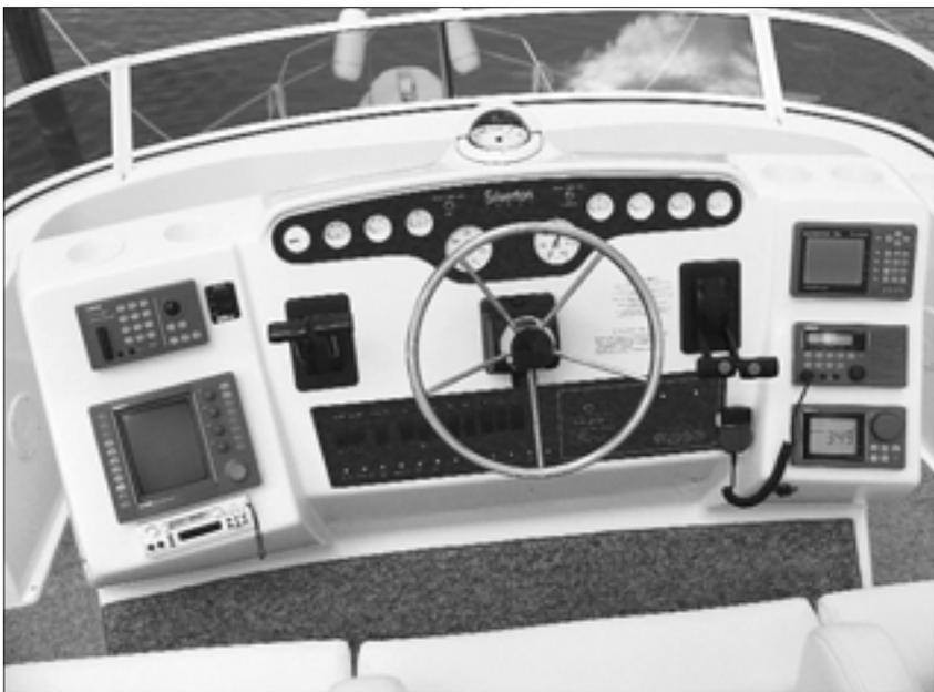
and "wing" instrument panels to either side. The wings are angled in towards the helmsman for better viewing of electronics.
